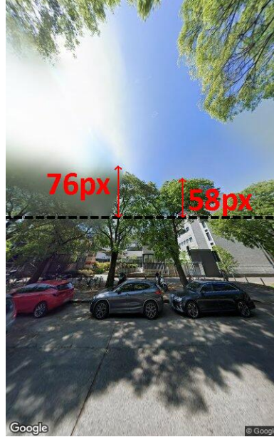
Fig. 5. Validating tree height calculations by measuring height above centreline. Image capture: Apr 2023 © 2025 Google, Italy.
